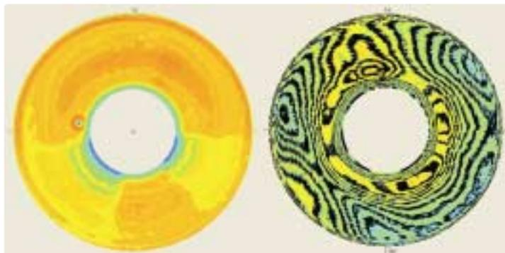
Figure 3: argusXE: (a) top view reveals SLT bump; (b) BD cover layer contour mapping
