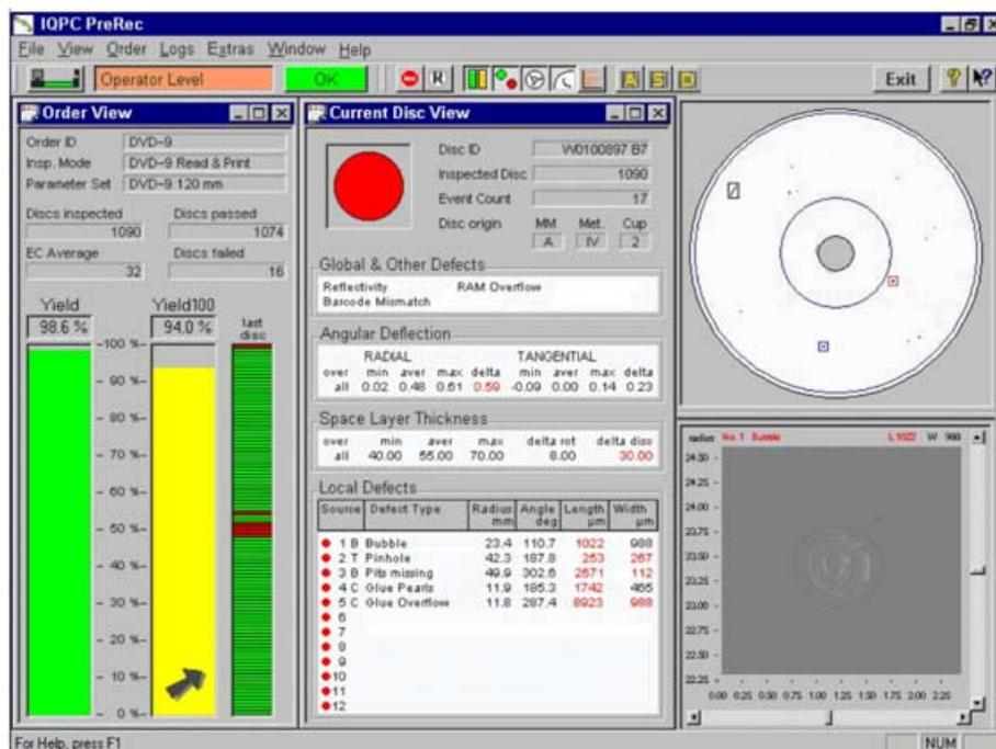
*Fig 1: Accurate defect detection and classification*
