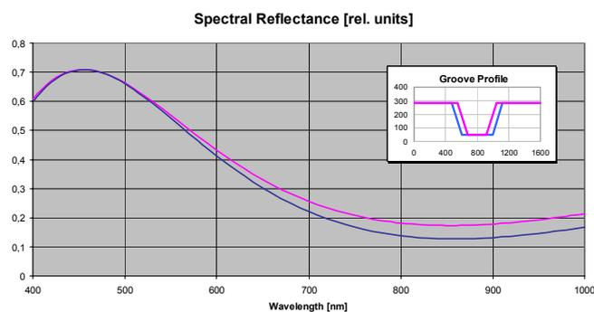
Fig 3b: Effect of width variation on zero order spectral reflectance
