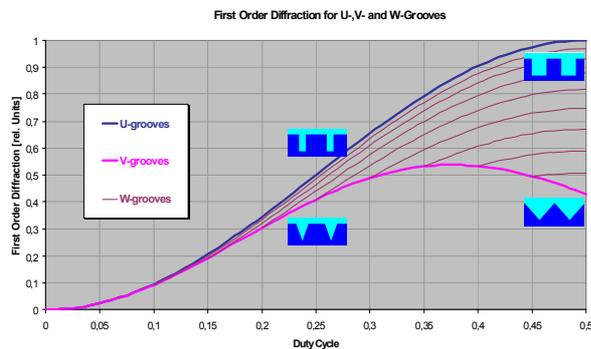
Fig 2a: First order diffraction as a function of duty cycle for U, V and W-shaped grooves
