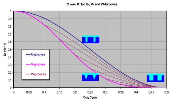
Fig 2b: Second over first order diffraction as a function of duty cycle for U, V and W-shaped grooves
