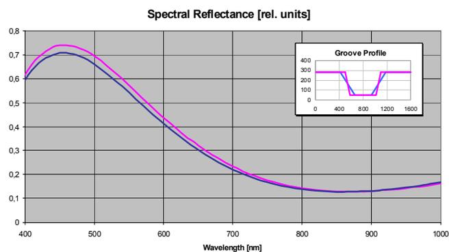
Fig 3c: Effect of wall angle variation on zero order spectral reflectance
