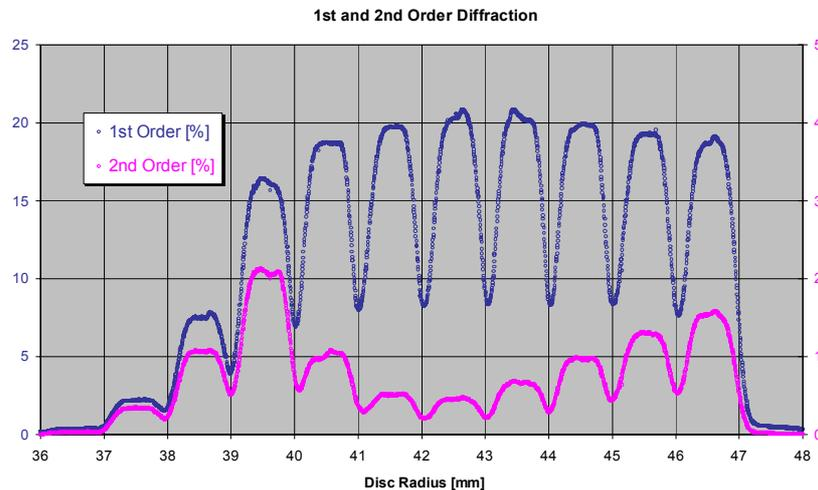
Fig 4a: First and second order diffraction measurements on a stepper master
