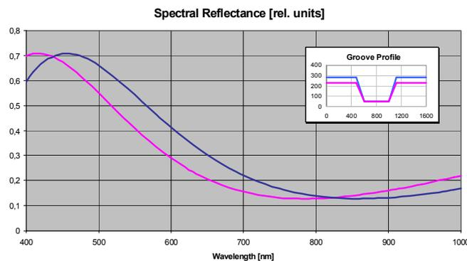
Fig 3a: Effect of depth variation on zero order spectral reflectance
