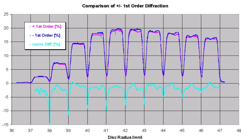
Fig 4b: Plus and minus first order diffraction measurements on a stepper master
