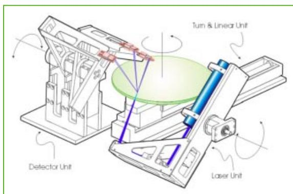
Figure 1 shows the diffraction order measurement module at the heart of the DOMS<sup>XE-blu</sup>, which supports a measurable track pitch range from 460nm to 2,000nm, with first order measurement down to 230nm. The system is designed such that there are no bearings or rails above the sample, eliminating the risk of abrasion or lubricant contamination. As an option, the system can be equipped with a downflow unit.
