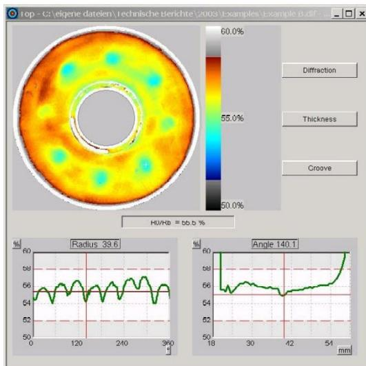
An example of stamper wear is given in Figure 6, which illustrates the importance of displaying the distribution of measurement results over the entire surface of the sample. The eight-point pattern indicates wear caused by injection flow and reflects the structure of the injection nozzle.
